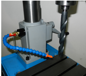
Magnetic Holder of Universal Bending Pipe (Able to stick to any metal surface) + Adjustable Water Valve
